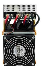
Connect the miner and the router by the Ethernet cable and then the miner can start to run after being powered on.
