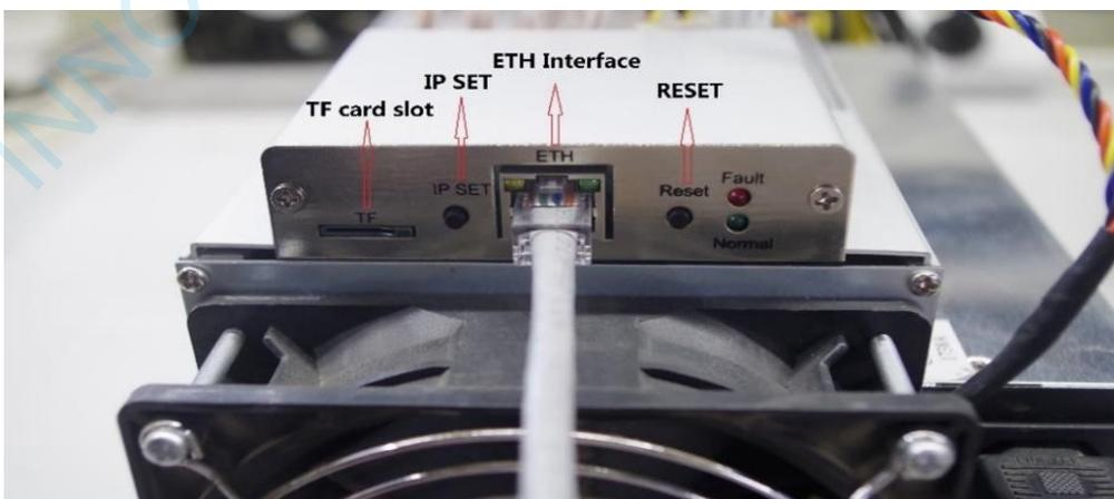
IP SET button: Press it more than 5 seconds to recover the IP to 192.168.1.254.
