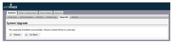
Choose 'Reboot' button, server will restart and run the new system. Choose 'Go Back', server will continue running the old system, will run new system when power on next time.
